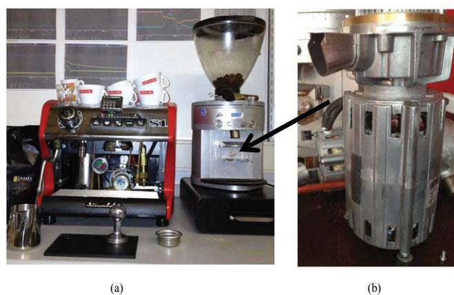
**Figure 4:** (a) Commercial espresso machine extraction and espresso coffee grinder (b) Grind chamber.
