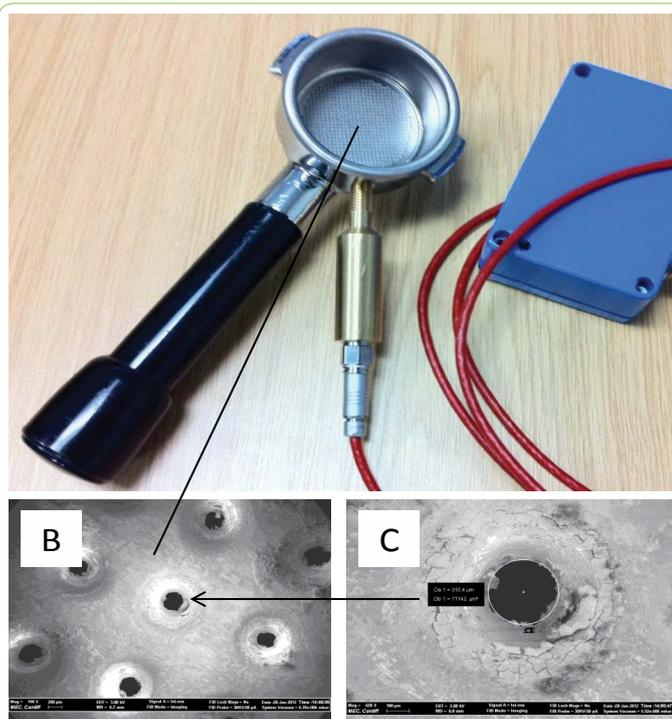
**Figure 6:** (a) Portafilter and coffee basket. (b) Coffee Basket holes (c) 336.6 μm Extraction hole size.
