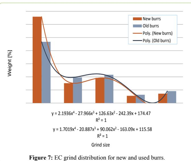
**Figure 7:** EC grind distribution for new and used burrs.
