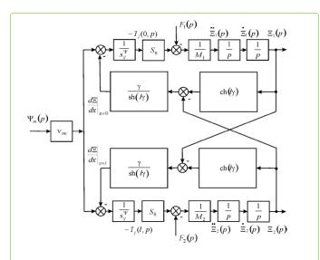
Figure 1: Generalized parametric structural schematic diagram of electroelastic actuator.
