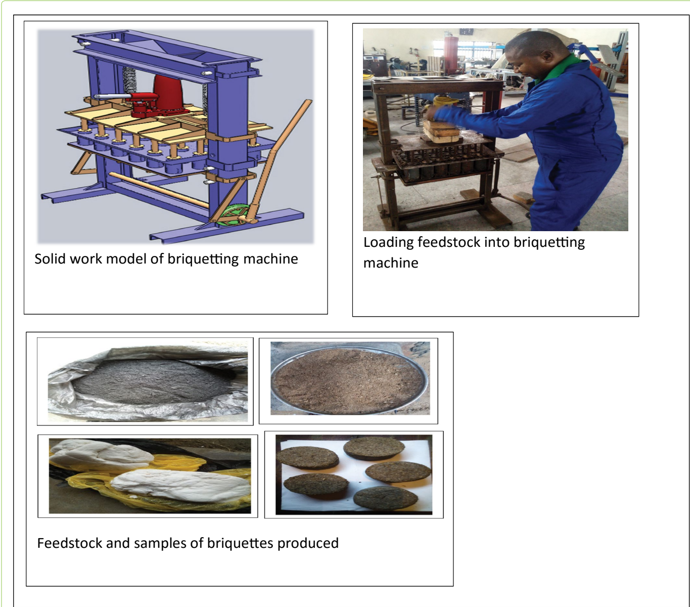
Figure 1: Solid work model, fabricated briquetting machine, feedstock and samples of briquettes produced.
