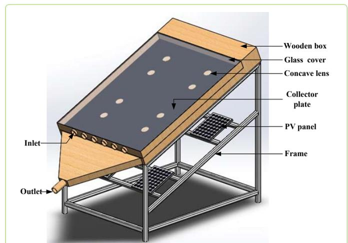
Figure 3: Isometric view of solar air heater with PV panel.
