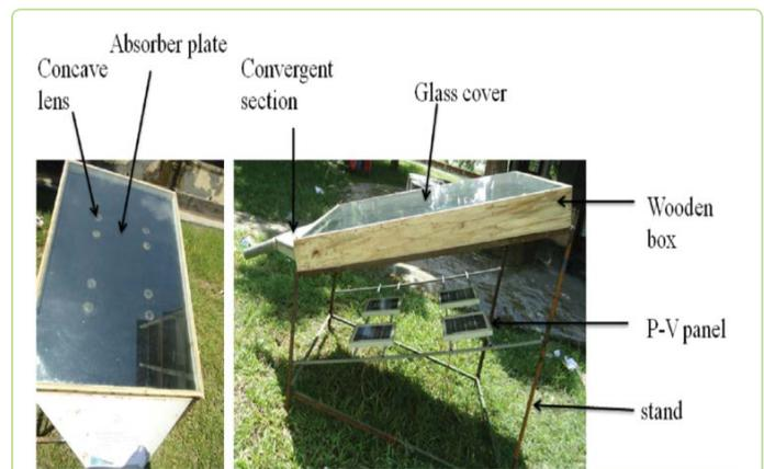
Figure 4: Final assembly of solar air heater.
