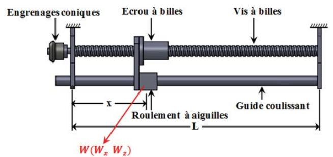
Figure 13: Mechanism of reconfiguration.
