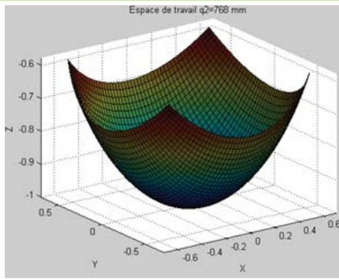
Figure 8: Workspace corresponding to the reconfiguration of  $q_2 = 768$  mm.
