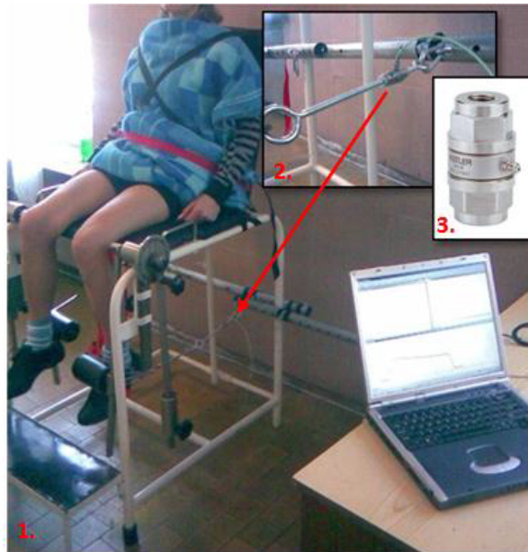
Figure: 1. Measurement of the maximum isometric muscle strength of knee extensors; 2. The measuring device and assembly structure; 3. Kistler force sensor (model 9311B)
